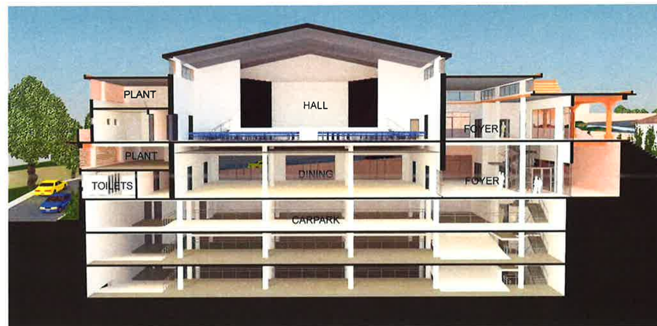
1 NORTH SOUTH CROSS SECTION (looking West)
